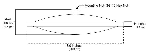
**TST429 Specifications:** • Continuous power handling: 135 watts • Impedance: 4 ohms • Overload Protection: Polyswitch • Frequency Response: 5Hz to 17kHz • Electrical Connecion: 3ft. - 16 guage, 2 wire • Dimensions: 8 in. diam. x 2.25 in. high • Recommended Amplification: 125 - 150 watts at 4 ohms • The TST429 is not approved for vertical mounting.
