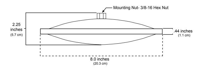
**TST329 Specifications:** • Continuous power handling: 135 watts • Impedance: 4 ohms • Overload Protection: Polyswitch • Frequency Response: 10Hz to 17kHz • Electrical Connecion: 3ft. - 16 guage, 2 wire • Dimensions: 8 in. diam. x 2.25 in. high • Recommended Amplification: 125 - 150 watts at 4 ohms
