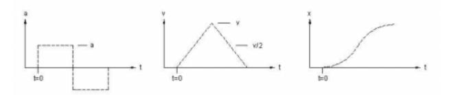
The conversion of electrical energy to kinetic energy is simple to examine when acceleration is constant and frictional losses are neglected. Consider accelerating a mass, m, at a constant rate, a, to final velocity, v, in time t. The force required to accelerate this mass is F, which equals ma. The energy required is the average power required times t. The average power required is the average velocity, v/2, times F. So the electrical energy required is
